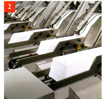
Stream feeding without bundle loading extension on flat pile feeder
