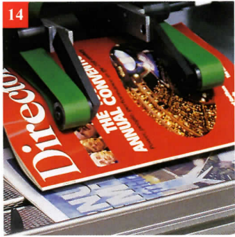
14 Inserting and film-wrapping unit Onyx/Rubin – for well-protected products with inserts of all types
